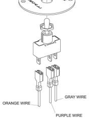
12. Fit the switch in to the opening, screw on the protective boot, and secure the switch with the nut from the other side of the panel.
