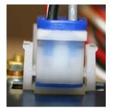
STEP 4: Push toward the other side so that the remaining locking tab clicks into a vertical position.
